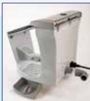
The suction hood is strategically located so that it doesn't obstruct. The hood is connected to an external suction tube at the rear through a pivotable outlet. Furthermore, detachable boxes collect the dust that could fall through the hand rests.
